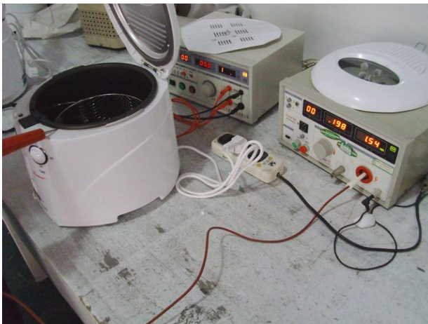
Hi-pot test at 4300V, 0.5mA 1s
