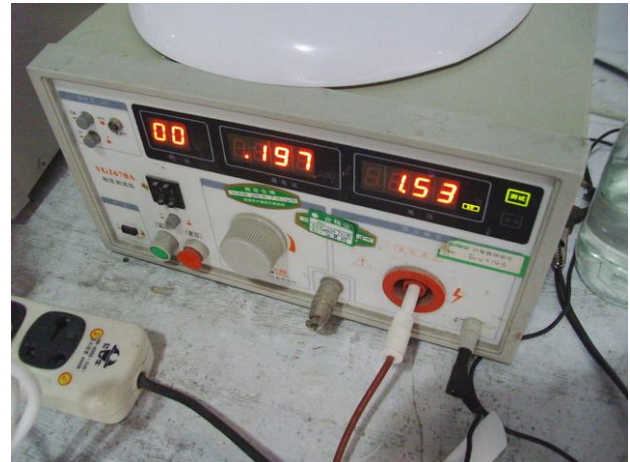
Hi-pot test at 1500V, 0.5mA 1s
